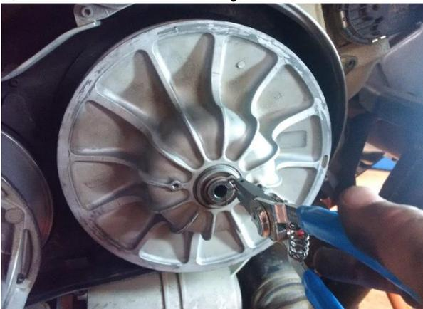
Remove the center bolt and the snap ring hold the friction washer. (photo 2017, serv. manual for updates)
