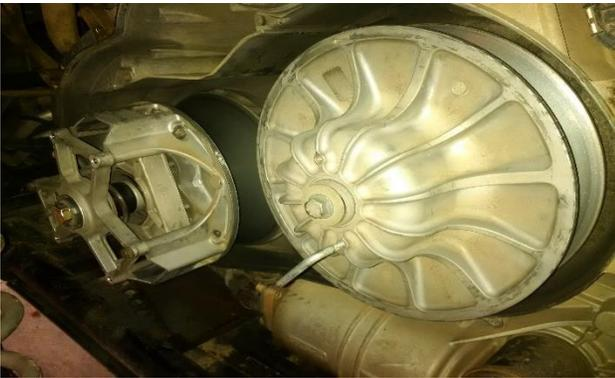
2) Take note of direction of belt before removal. Remove belt.
