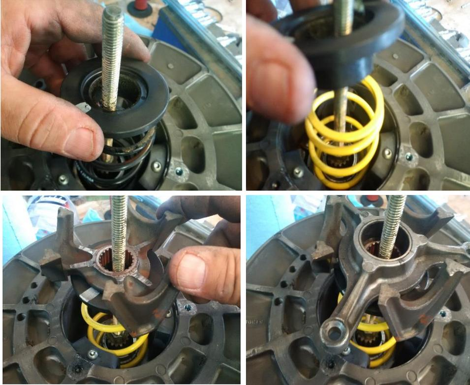
10) Take notice of the spring spacer, spring, and helix, then remove the stock secondary spring, and replace it with the spring provided.
