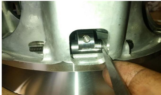
With stock clutches it is very common to see the side of the clutch wearing from the flyweight pivot end gouging into the aluminum, even with only low miles.
